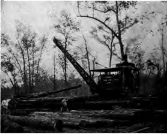
FIG. 92. — A Model C American Log Loader.
